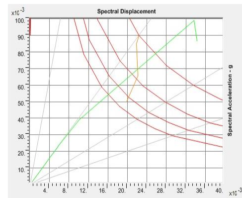
Fig. 4 Capacity Spectrum for Model 2 (L Type shear wall at corner)
