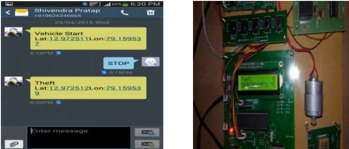
Figure-6: DC Motor stops as 'STOP' message is received
