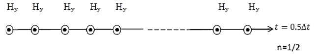
Figure 3.2 1D space-time chart of the Yee algorithm showing central differences for the space derivatives and leapfrog over the time derivatives, k represents electric field node numbers and n is the time step[18]
