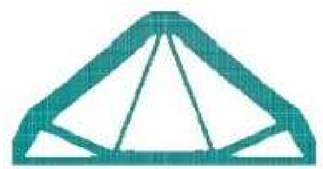
Fig.4: Optimal design for Model 1 by BESO method
