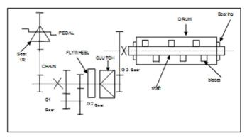
Figure-1: Schematic arrangement of a Nursery Fertilizer mixer machine.
