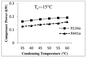
Fig. 3 Compressor Power Input vs Condensing Temperature
