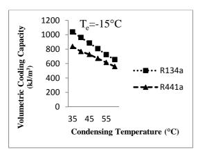
Fig. 2 VCC vs Condensing Temperature
