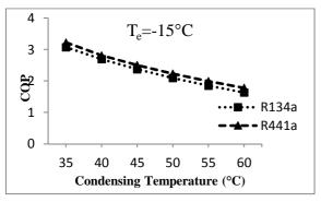
Fig. 1 COP vs Condensing Temperature
