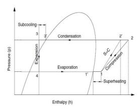
Fig.1 (b) Pressure – enthalpy (P-h) diagram of Vapour Compression refrigeration cycle.
