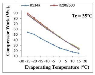
Fig.3 Variation of Compressor Work  $(W_C)$  with varying Evaporating Temperature
