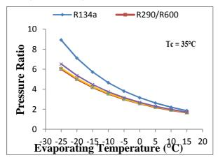
Fig.2 Variation of Pressure Ratio (PR) with varying Evaporating Temperature.
