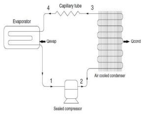
Fig.1 (a) Schematic Diagram of Vapour Compression refrigeration Cycle
