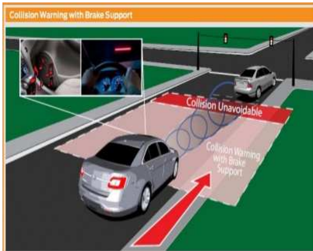
Figure 4: situation showing collision warning with brake support.
