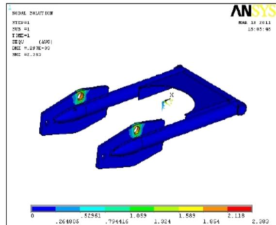
Fig. 2.3 Structural analysis of suspension frame using aluminium alloy a360
