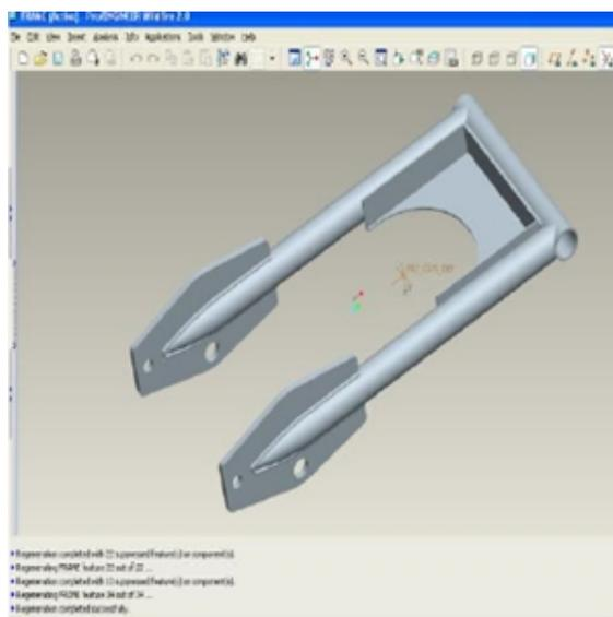
Fig. 2.2 Pro/Engineer model of suspension frame
