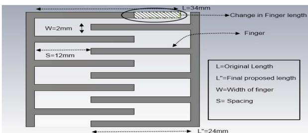
Fig.1: Proposed Interdigital filter structure
