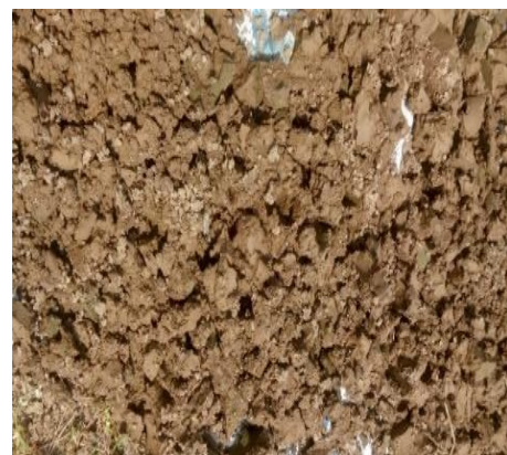
Fig no.2- Collected water treatment plant sludge
