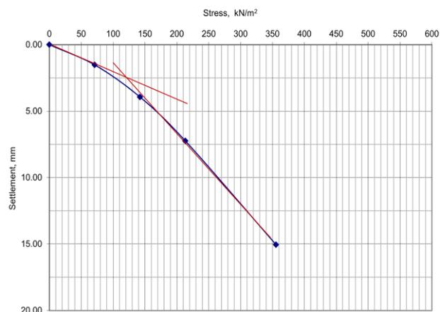
**Fig. 5:** Stress-settlement curve for test location PLT-01
