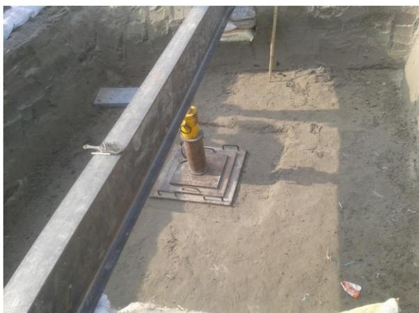
**Fig. 4:** Test Pit Arrangement for Plate Load Test
