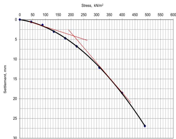
**Fig. 6** Stress-settlement curve for test location PLT-02
