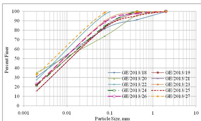
**Fig. 9:** Grain Size Distribution Curves
