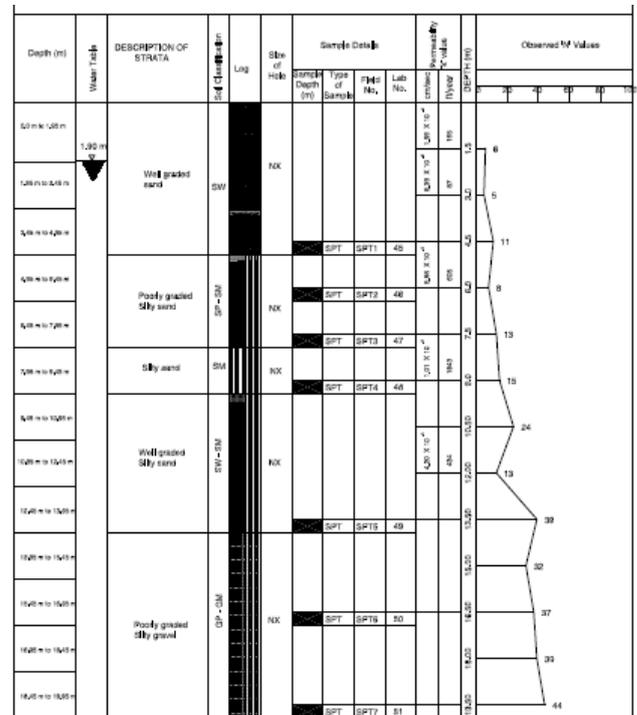
**Fig. 2:** Log of bore hole [3]
