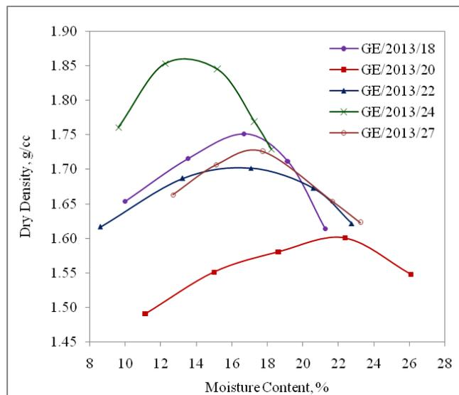
**Fig. 10:** Compaction Curves
