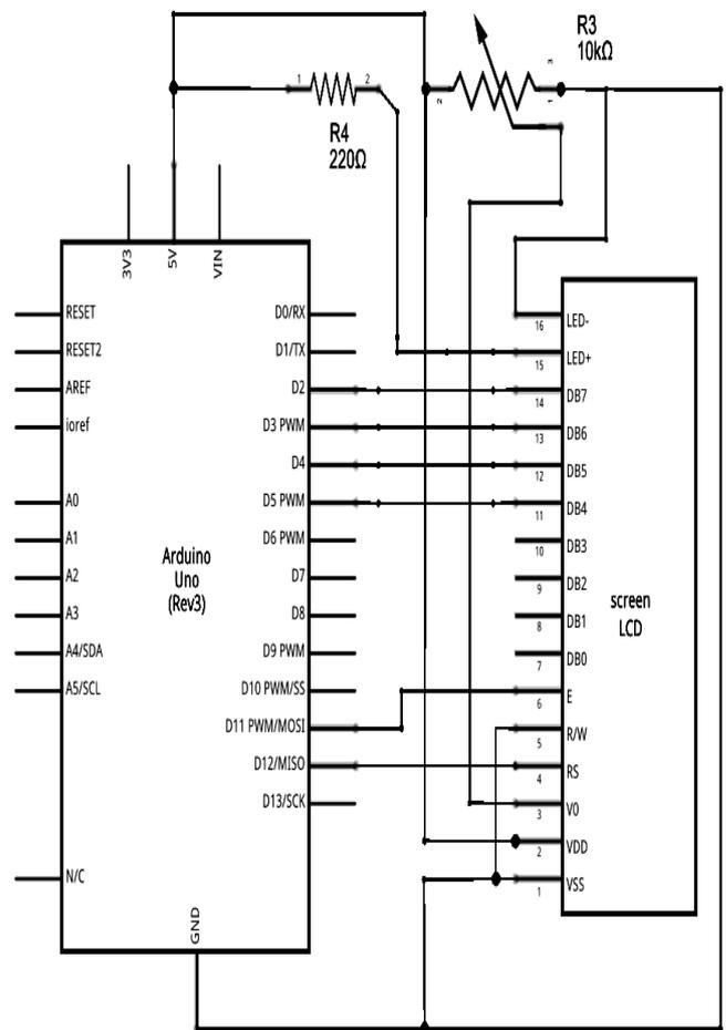
Fig 3.5 LCD Interfacing with Arduino
