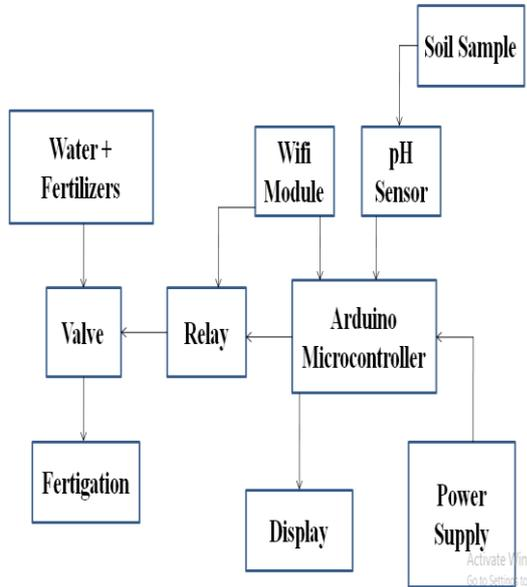
Fig.2.1 Block diagram
