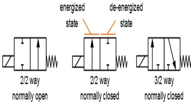
Fig 3.8 Valve circuit functions
