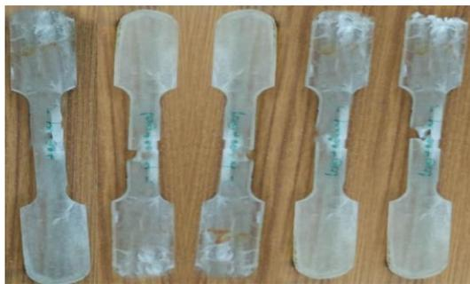
Figure 7. Sample after tension test
