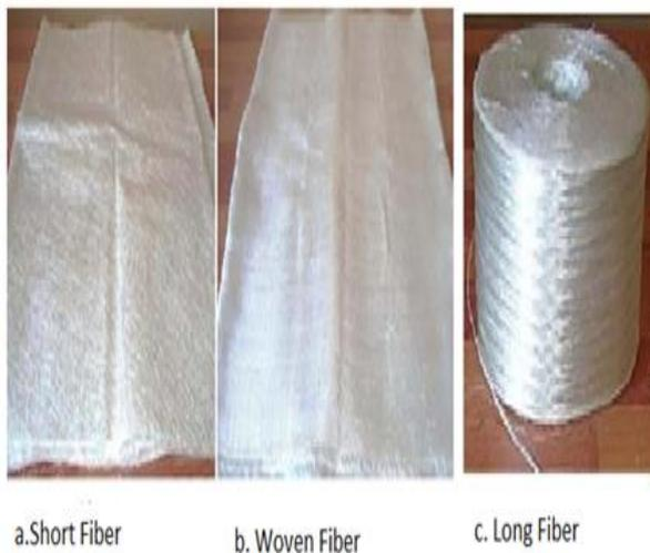
Figure. 1. Over view pictures for types of composites fiber.
