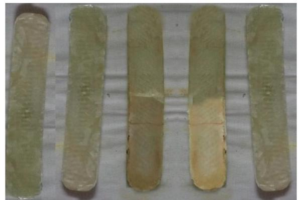
Figure 10. Specimens of woven fiber after tension test
