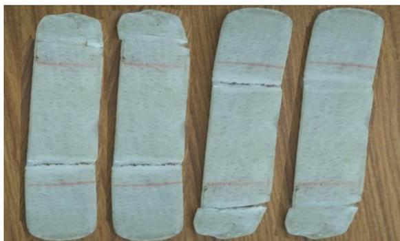
Figure 9. Specimens of long fiber after tension test
