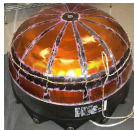
Fig 1: A cylindrical pressure vessel with toroidal end caps
