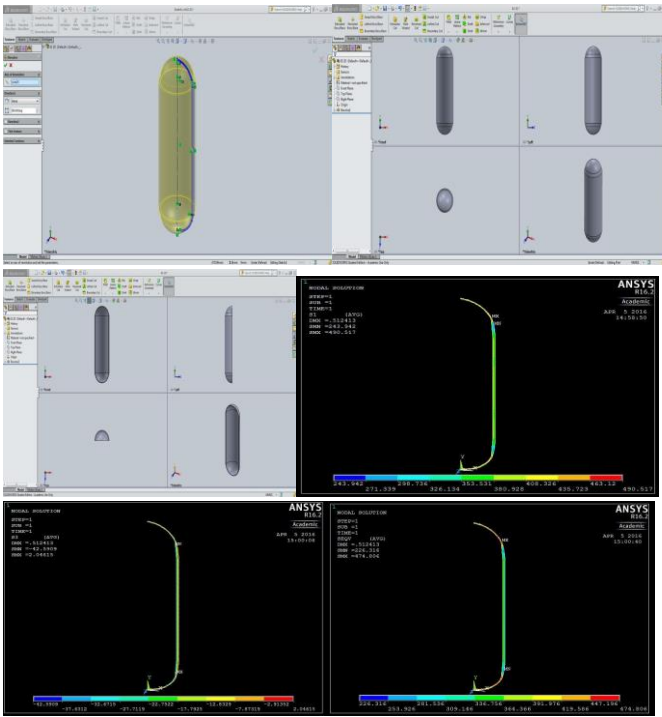
Fig 5-12 Design og Pressure vessel of 63 mm diameter
