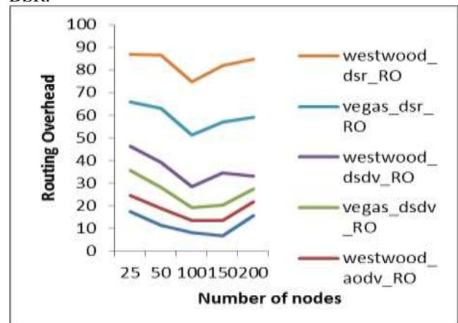
Figure 5.5: Illustrates routing overhead vs. number of node
