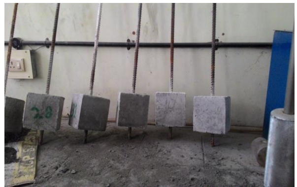
Fig 3.2.1. View of Bond strength Test Specimen after cement capping
