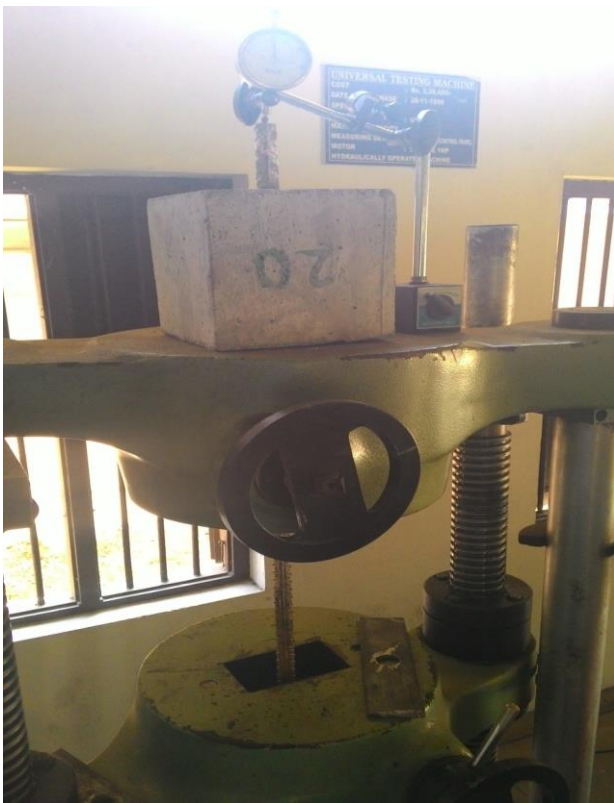
Fig.3.3.1. Arrangement of pullout test in UTM
