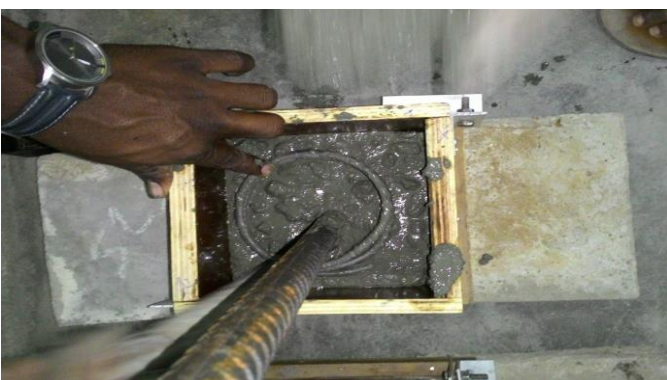
Fig 3.1 Arrangement Inside The Mould For Bond Strength Test Specimen
