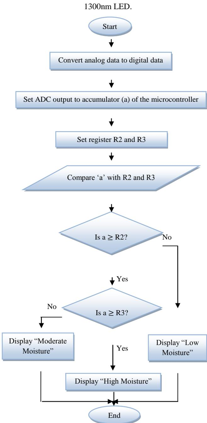
Fig-9: Flowchart for microcontroller programming.
