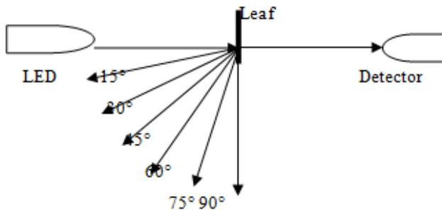
Fig-1: Set-up for transmittance and reflectance measurement.
