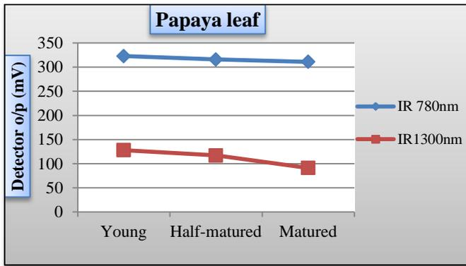
Fig-5: Transmittance characteristics for LED are of wavelength 780 nm and 1300nm.
