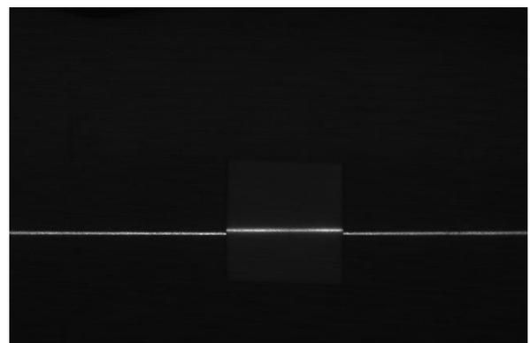
Fig-3: Deviation in laser line due to presence of object
