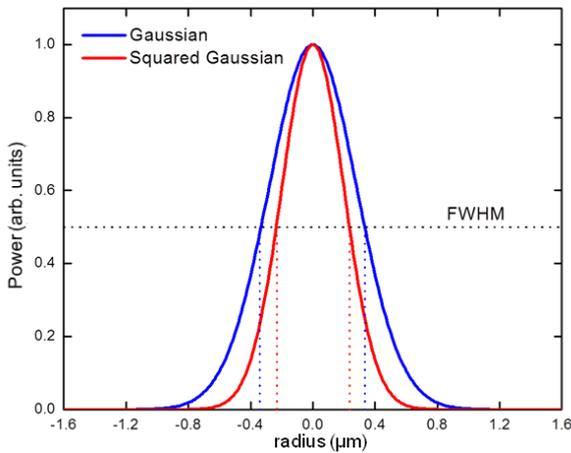
Fig-6: Power distribution profile of a laser
