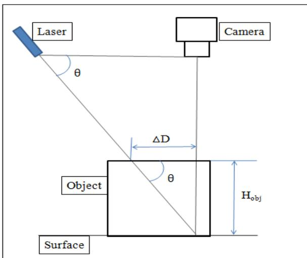
Fig-2: Laser triangulation geometry in presence of object
