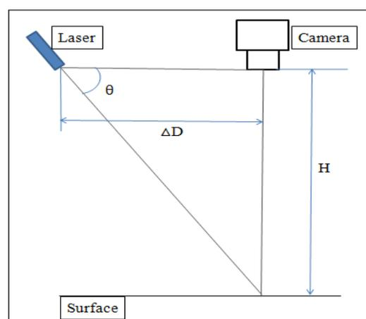
Fig-1: Laser triangulation geometry
