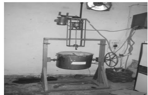
**Figure 2:** Tilting resistance furnace used for production of Al-SiC foam.
