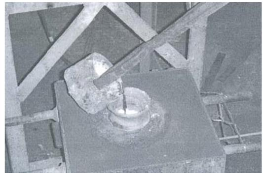
**Figure 1:** Pouring of Al-SiC melt into mold.
