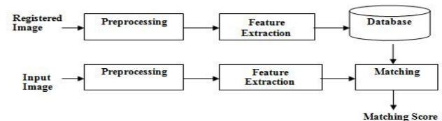
Fig 3. Flow diagram of biometric recognition system
