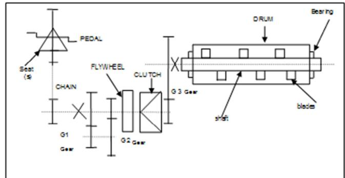
Figure-1: Schematic arrangement of a Nursery Fertilizer mixer machine.
