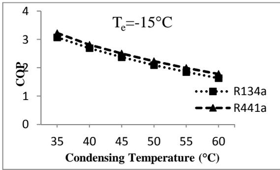
Fig. 1 COP vs Condensing Temperature
