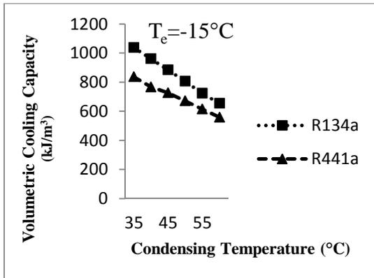
Fig. 2 VCC vs Condensing Temperature
