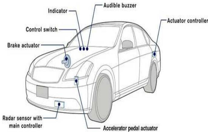
Fig-2: Structure of the system<sup>[5]</sup>
